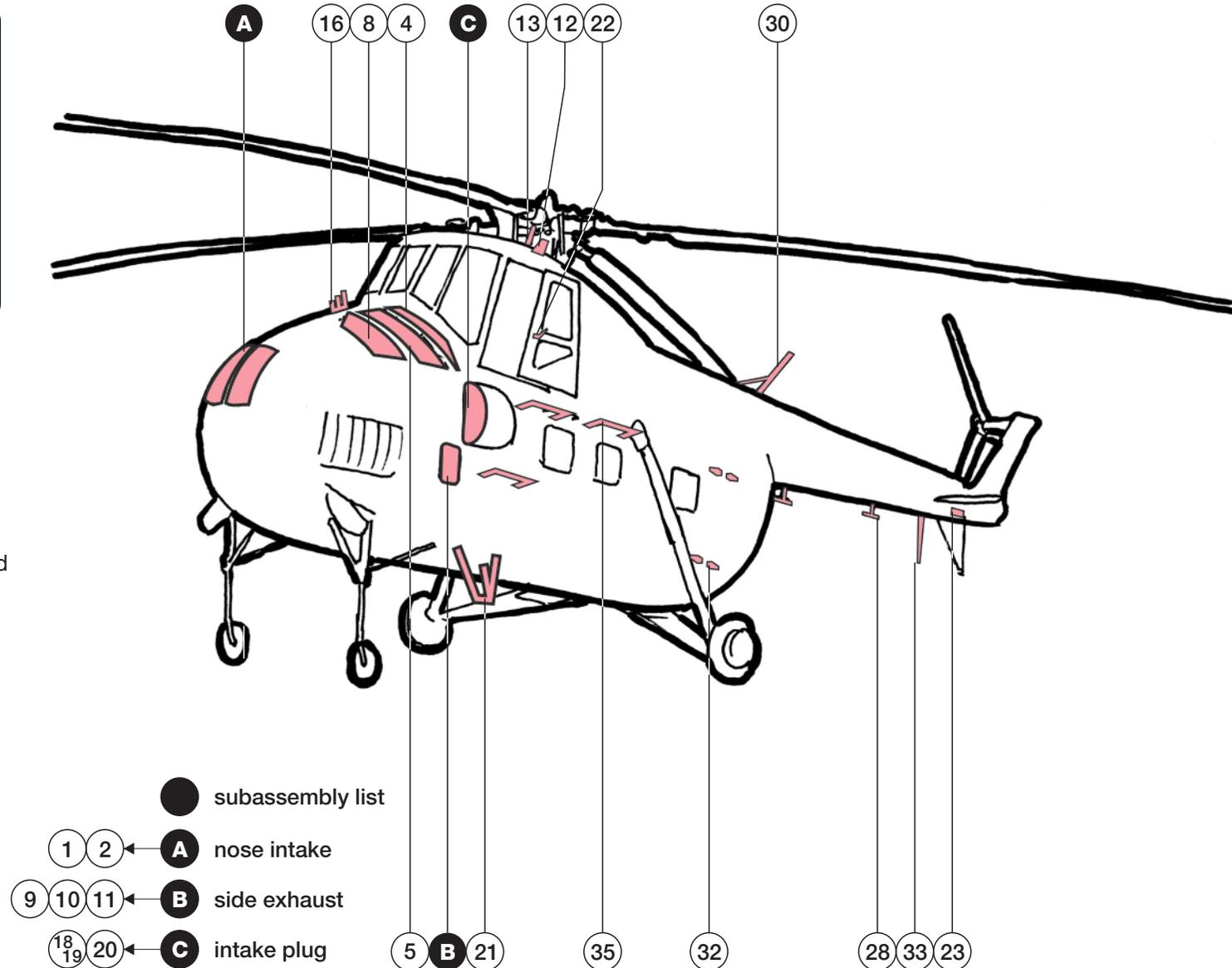
Nose inlet (A) and side exhaust (B) are sandwich affair. Side exhaust is easy – put part 11 on top of part 10, and add part 9 to the bottom of part 10. This sub-assembly should be set about 0.5mm inside fuselage part, and can be later surrounded by additional collar made of 0.7–1mm wide strip of aluminum foil.
