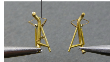
main gear struts scratch built from brass tubing
