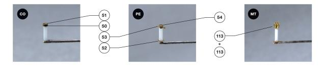
As a column of compass (CO), pelorus (PE) and the machine telegraph (MT) use 1.6 mm long pieces of Ø 0.3 mm plastic rod.
