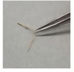
Small (narrow) tripod legs are relatively easy to fold. Large tripod legs are trickier to fold evenly. First press the back of fold line with the blade until the halves are at about 135° to each other (top photo). Then follow the fold gently until about 90-80° using your fingers. In the final stage use tweezers positioned as shown on bottom photo - the halves should snap together, regiuiring just a hint of CA glue at the tips to hold them together.
