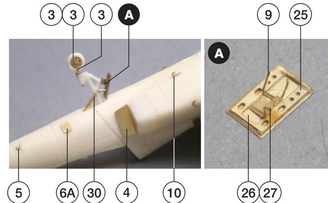
Catapult hooks (10) and pitot (28) feature small nib, which coupled with hole in fuselage (use 0.25mm drill bit) results in much stronger joint and easier positioning.
