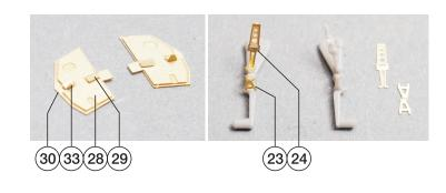
Front gear diagonal strut (3) comes with approach light that is missing in plastic part. You can consider leaving out part 19 and keeping the kit strut, this will help to keep the geometry.
