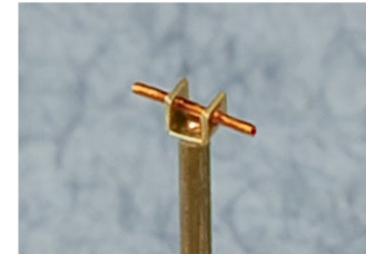
Double reinforced joint made using SO5720009 set.
