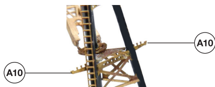
Location of the signal lines supports on the main mast.
